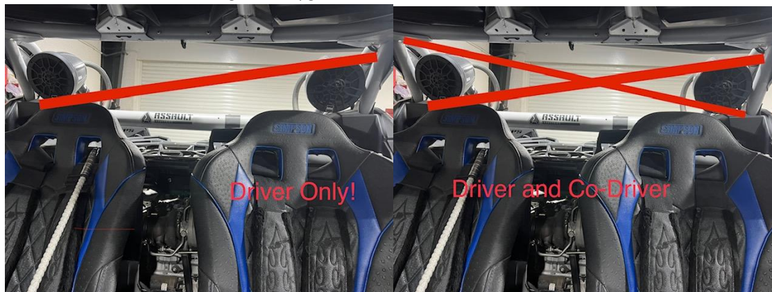
Pic 17.1 Example of main roll bar brace for both driver and driver/co-driver configuration.
