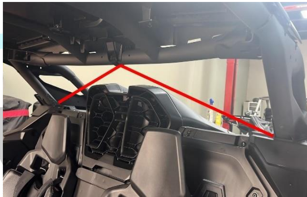
Pic 17.1 Example of main roll bar brace for both driver and driver/co-driver configuration.
